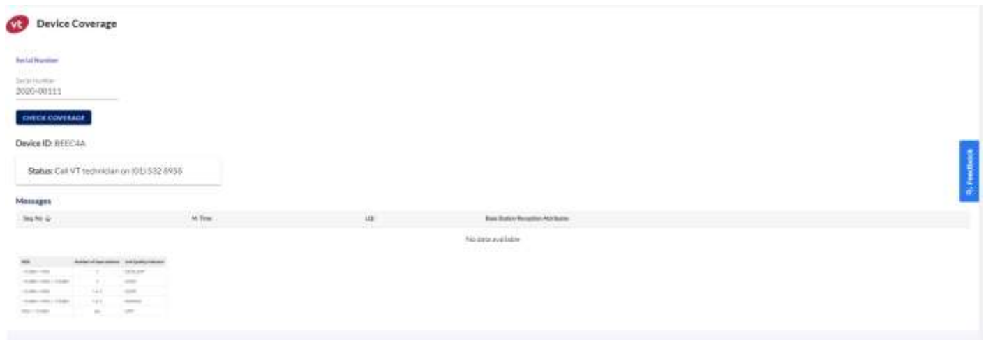
FIGURE 31: VT IoT INSTALLATION AIDE WEB APPLICATION USED BY INSTALLERS TO VERIFY ON SITE COVERAGE AND CORRECT INSTALLATION
