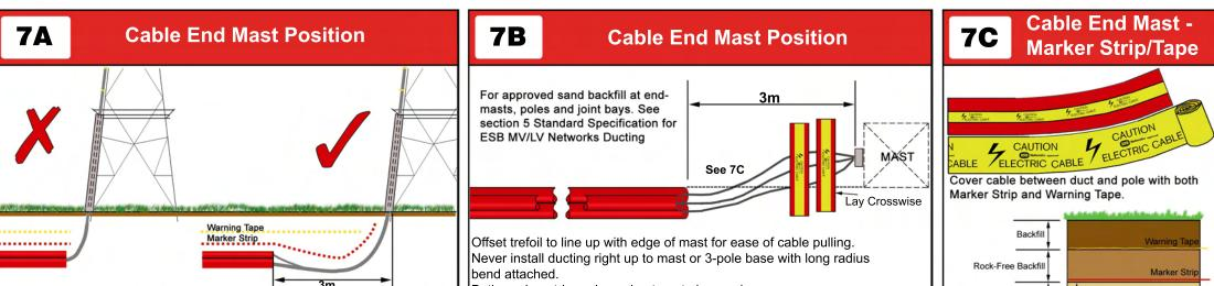
Ensure that trench is deepened at this position and cable is supported all round so that it does not tighten further during Backfilling Both marker strip and warning tape to be used between duct and mast (laying the marker strip crosswise as shown above).
