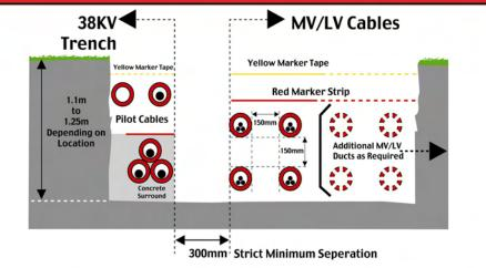
Where it is impractical to avoid such trench runs, the seperation of 300mm should be strictly controlled and monitored to minimise derating (See MV/LV manual page 180)
