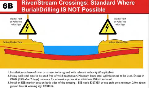
4. Ensure a smooth connection using rubber coupler between crossing pipe size and ESB standard duct as the steel pipe size will usually differ from the standard ESB ducting. Alternatively run ESB ducting right through the steel pipe
