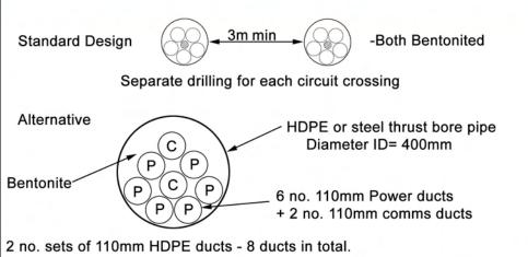
All crossings to be accurately recorded and signposts erected given impracticality of marker tape. If both circuits = 40MVA then use 630 Cu cable
