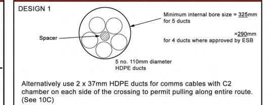
Completed interstitial space to be bentonited thoroughly to maintain cable rating. Accurately record crossing location & erect marker posts.
