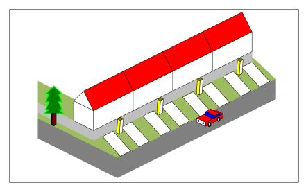
Figure 1 Parking and EV Chargepoints in housing estate layout without off-street parking
