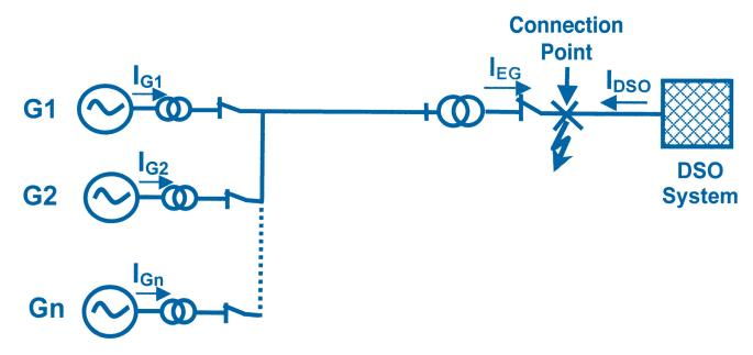
Legend: **EG:** Fault Current Contribution from Embedded Generation Facility **IDSO:** Fault Current Contribution from DSO System **IGn:** Fault Current Contribution from Individual Generation Unit
