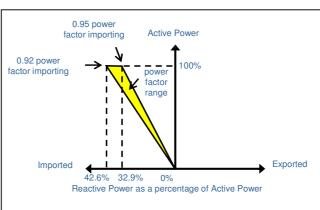
The new diagrams necessary show lines going through the origin, which means PF is maintained at all MW levels.
