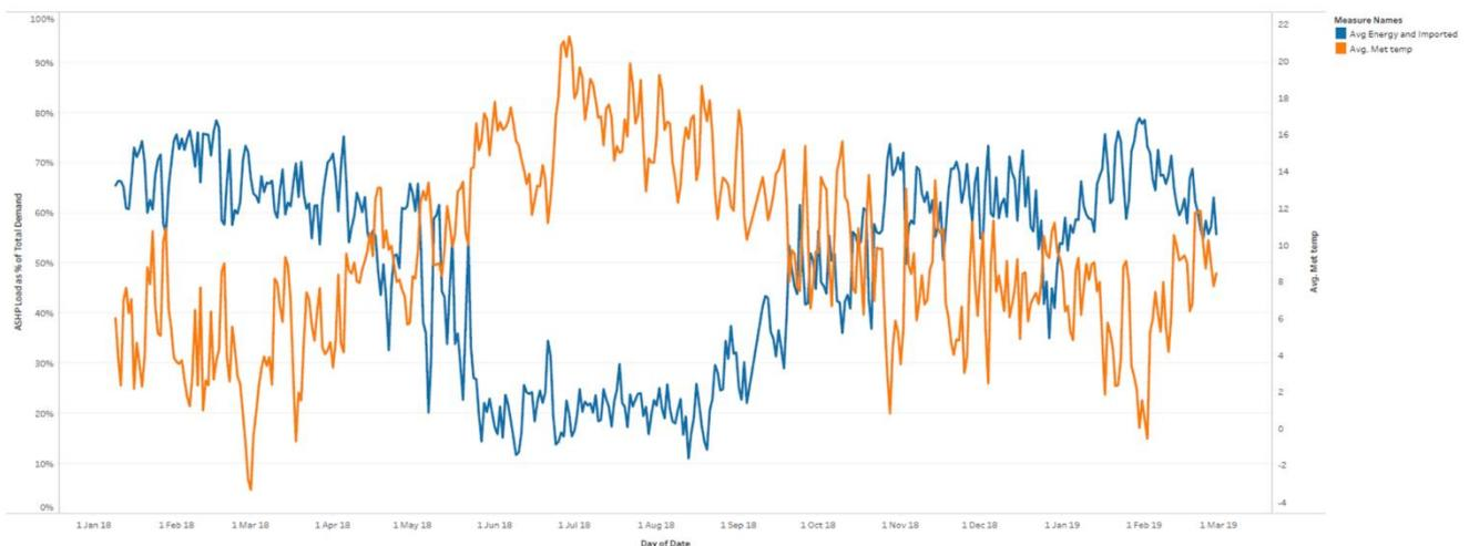
**FIGURE 3: AVERAGE ELECTRICAL ENERGY IMPORTED (BLUE) VS AVERAGE METEOROLOGICAL TEMPERATURE (ORANGE) FOR THE FLEET OF SUPERHOMES OVER THE PERIOD JANUARY 2018 TO MARCH 2019.**
