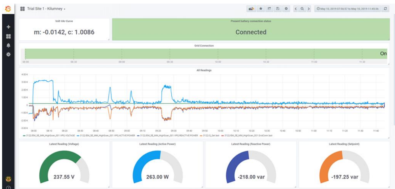
FIGURE 3: CONTROL & MONITORING PLATFORM SHOWCASING REACTIVE POWER SET POINT TRACKING AT A BATTERY TRIAL SITE
