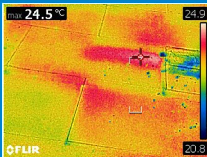
Figure 3.5: Thermal Fault Hotspot
