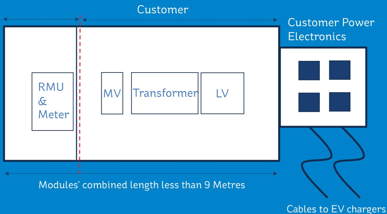
Figure 3.3: MV/LV Modular Substation – EV Charging
