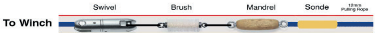
Fig 11B - Set up for Swivel, Brush, Mandrel and Sonde for Duct proving and Cleaning
