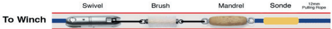
Fig 11B - Set up for Swivel, Brush, Mandrel and Sonde for Duct proving and Cleaning
