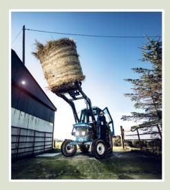
DO take extreme care when moving objects or loads near overhead wires. In general, keep long items in a horizontal position when moving them.
