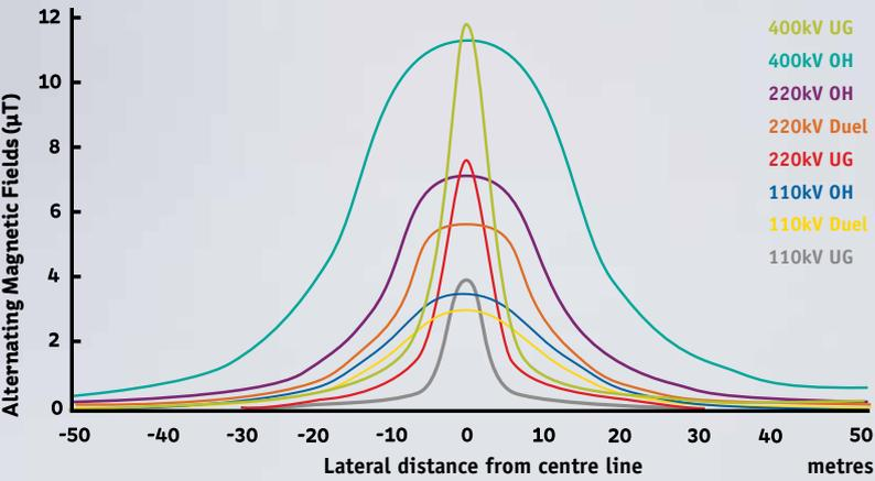
**Figure C** illustrates the magnetic field from overhead AC lines operating in Ireland. The field strength decreases with distance. The fields from these AC lines are far below the 1998 ICNIRP Guidelines for exposure to AC magnetic fields (100µT). In 2010 ICNIRP updated its ELF-EMF guidelines, which included the recommendation for a 200µT reference level for exposure for the general public, but these have not yet been adopted by the European Union.
