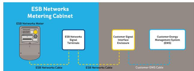
**Figure 1:** Customer signals equipment layout Signal Information
