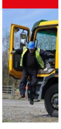
Shuffle away from the vehicle. Take half steps only or hop with both feet together to minimise the possibility of electric shock
