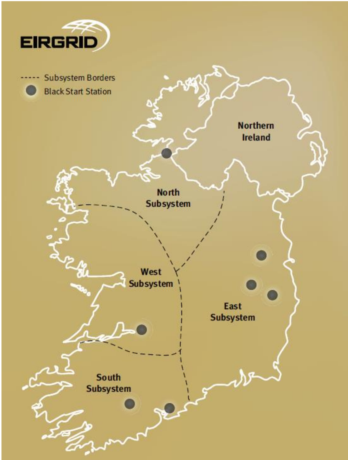
Figure 1- Simplified overview of Black Start Stations and Subsystem Borders
