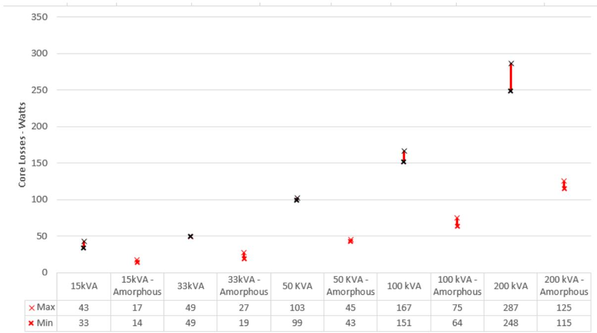
**FIGURE 1. GUARANTEED CORE LOSSES FOR CONVENTIONAL AND AMORPHOUS CORE TRANSFORMERS**
